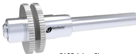
SAPE Arbor Shown. Included Spacers Allow For Double Saw Configuration.
